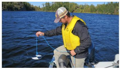
Figure 2 - Lowering of Secchi disk
