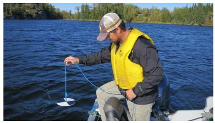
Figure 2 - Lowering of Secchi disk
