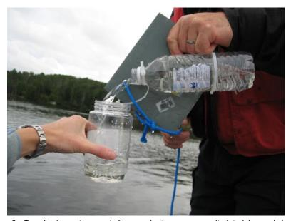
Figure 3 – Transferring water sample from euphotic zone composite into lab sample bottle
