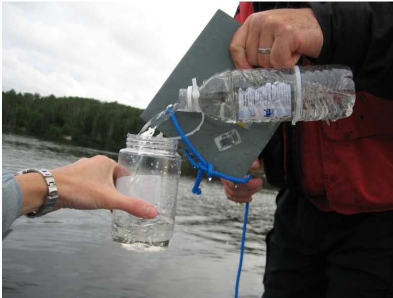
Figure 3 – Transferring water sample from euphotic zone composite into lab sample bottle
