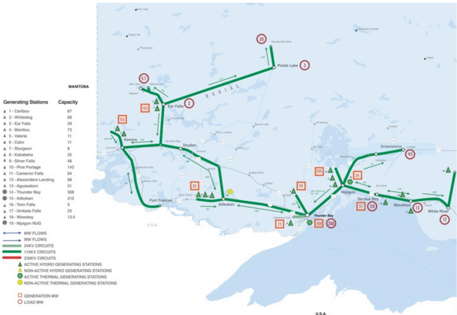
Figure 9 115 KV Distribution System (arrows show direction electrons can and do move as required)
